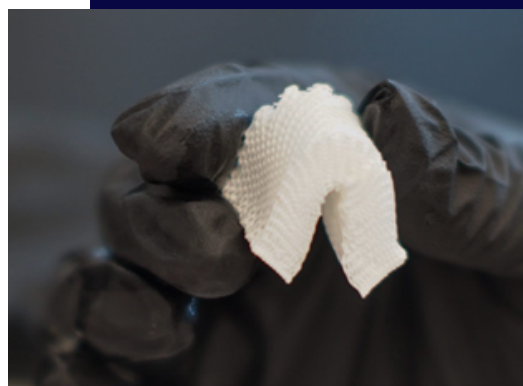
Flexibility after 15 minutes of submersion in fluid at about 37°C
